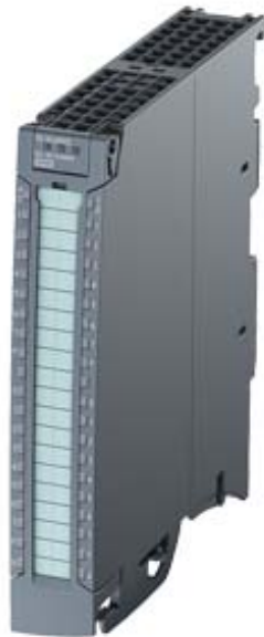
SIMATIC S7-1500, DIGITAL OUTPUT MODULE, DQ 32 X 24VDC/0.5A; 32 CHANNELS IN GROUPS OF 8, 4 A PER GROUP; INCL. FRONT CONNECTOR PUSH-IN
