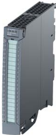
SIMATIC S7-1500, DIGITAL OUTPUT MODULE, DQ 16 X 24VDC/0.5A; 16 CHANNELS IN GROUPS OF 8, 4 A PER GROUP; INCL. FRONT CONNECTOR PUSH-IN
