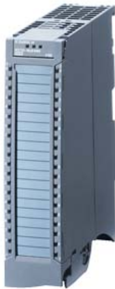
SIMATIC S7-1500, DIGITAL INPUT MODULE DI16 X AC230V, 16 CHANNELS IN GROUPS OF 4; INPUT DELAY 20MS; INPUT TYPE 1 (IEC 61131)
