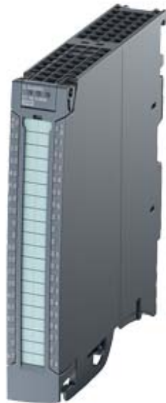
SIMATIC S7-1500, DIGITAL INPUT MODULE, DI32 X DC24V, 32 CHANNELS IN GROUPS OF 16; INPUT DELAY TYP. 3.2MS; INPUT TYPE 3 (IEC 61131) INCL. FRONT CONNECTOR PUSH-IN
