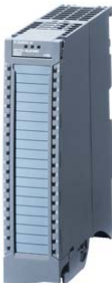
SIMATIC S7-1500, DIGITAL INPUT MODULE DI16 X DC24V, SOURCE; 16 CHANNELS IN GROUPS OF 16; INPUT DELAY 3.2MS; INPUT TYPE 3 (IEC 61131)
