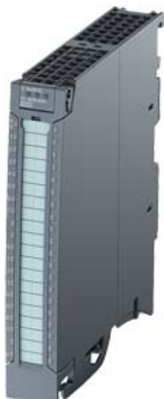
SIMATIC S7-1500, DIGITAL INPUT MODULE, DI16 X DC24V, 16 CHANNELS IN GROUPS OF 16; INPUT DELAY TYP. 3.2MS; INPUT TYPE 3 (IEC 61131) INCL. FRONT CONNECTOR PUSH-IN
